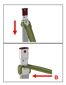
2.Pull down head piece while buckle is pressed.
