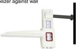
2. Hitching the measuring tape to the lower hook at slider when use without scale.
