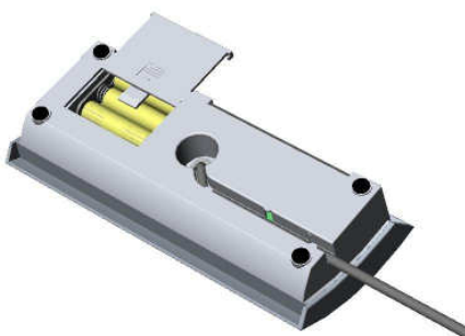
6. Reinstalling the battery cover.
