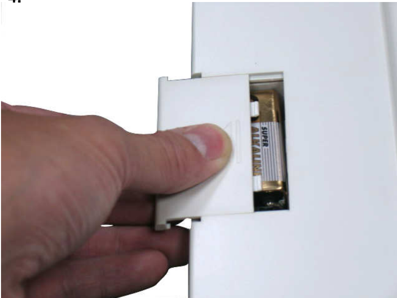
INSTALLING BATTERY COVER
