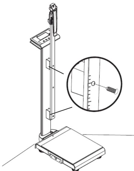
\*Screw the height rod on the bracket.
