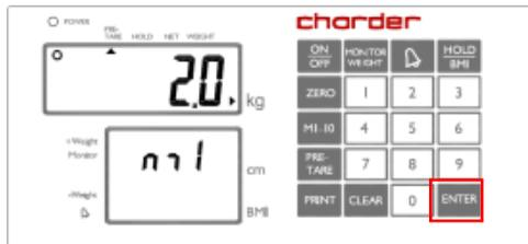
**NOTE:** Pre-tare weight must be under max capacity, otherwise screen will show 0.00 after **ENTER** key is pressed, and the operator will have to re-input pre-tare settings.
