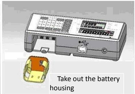
3. Use either rechargeable battery pack, or AA batteries
