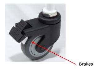
2. To tighten wheel castor, loosen counternut slightly. After loosening, turn wheel frame clockwise to tighten.
