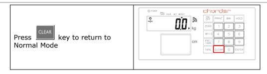
NOTE: Pre-tare weight must be under max capacity, otherwise screen will show 0.00 after key is pressed, and the operator will have to re-input pre-tare settings.
