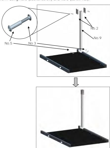
2. Assemble pole on platform using same procedure as Step 1.
