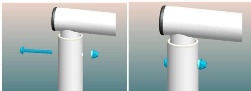
**NOTE:** securely tighten screws mounting handrail to column.
