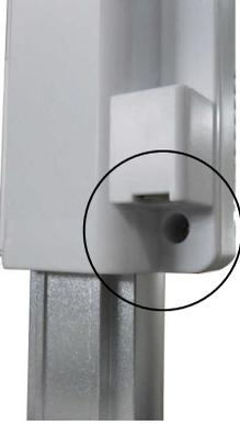
2. Connect USB cable (9 pin DIN) to USB port on height rod.
