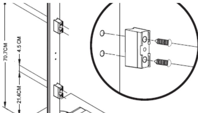
2. Attach height rod to fixing blocks using two screws.
