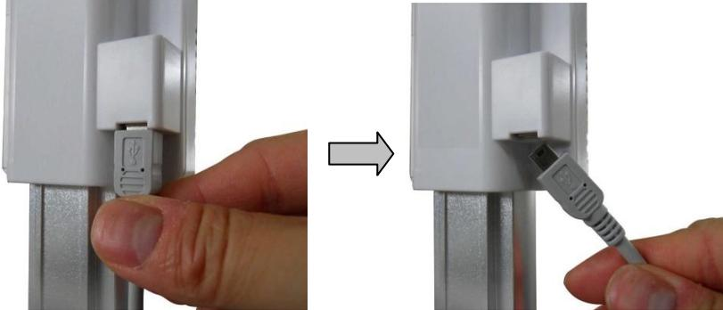
3. Locate 9 pin DIN port on bottom of indicator, and connect USB cable.
