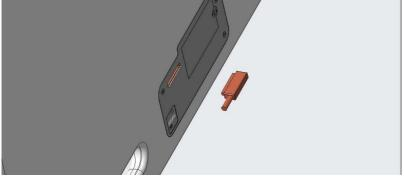
The port for the charging cable is magnetic. Clip end of cable in place, and plug other end of cable into power mains. Device cannot be used while charging. Do not use any form of charging cable other than the one supplied with the device.
