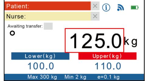
**\*NOTE:** If the Weight Tracking Function is activated, the original subject's weight will be saved in memory. This function can be activated only after the bed has been pushed onto the weight bridges, and the subject is lying down on the bed.
