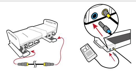
**Note**: connect both weight bridges to one another using weight bridge connecting wire. Connect indicator to weight bridge 2 (blue port).
