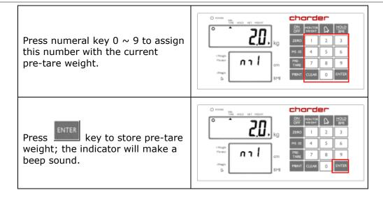
**NOTE**: Pre-tare weight must be under max capacity, otherwise screen will show 0.00 after key is pressed, and the operator will have to re-input pre-tare settings.
