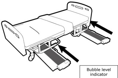
2. Device should be placed on non-slippery, flat, hard, level surface. Make sure bubble level indicator is centered to ensure result accuracy.
