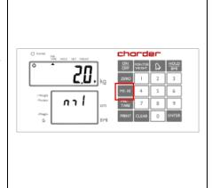
**Note**: If total weight exceeds scale capacity (includes tare), indicator will display "Err" prompt due to overload.
