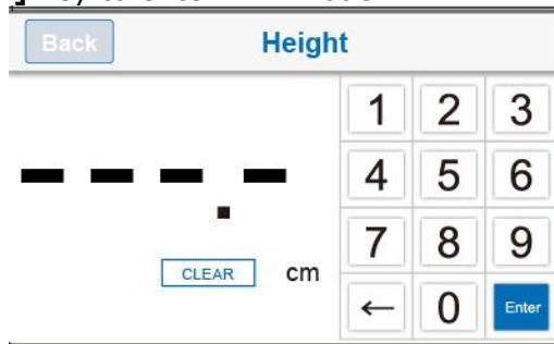
2. Enter height using numeral keys (ex: to input 170 cm, press 1-7-0-0). Press **[CLEAR]** key to re-input.
