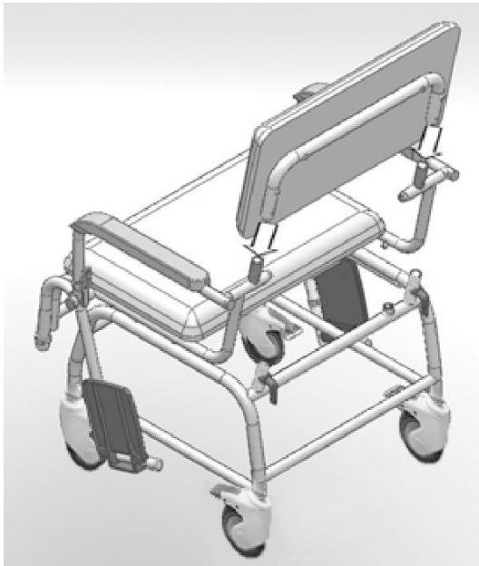
3. Insert E-type clips into hole to secure backrest
