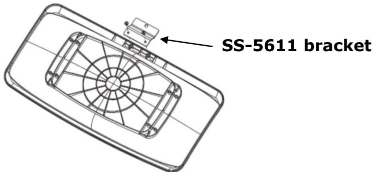
2. Slide HM80M onto bracket, and press buckle to secure
