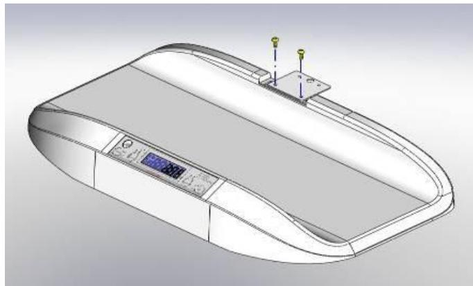
3. Attach height rod to bracket carefully until a click noise is heard.
