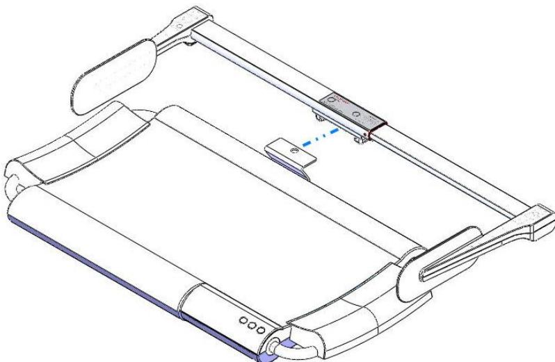
3. To detach height measure, find the latch located at the rear of the attachment. Press down on the buckle, and gently remove the attachment from bracket.
