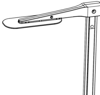
4. Install height rod + headstopper onto bracket using Philips screws
