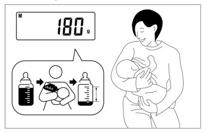
Milk Intake function will always store current weight which is placed on the tray and deduct last stored weight and display the differences.
